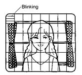
Move the cursor to the area where backlight is bright and press it to mask that area. The mask turns white. (When the cursor is moved on an area that has already been masked, the mask and cursor start blinking.)
